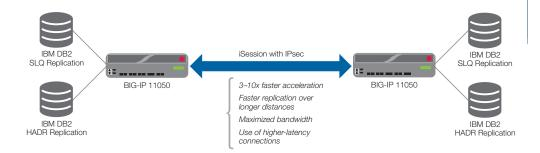
BIG-IP acceleration technology significantly improves throughput of IBM replication and any other cross-data center traffic
